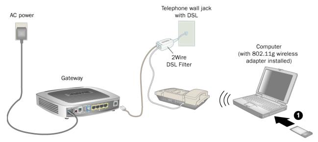
Figure 6. Gateway Connected to Second Computer Via Wireless
